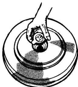
1 Removing Arming Plug From Mine.
